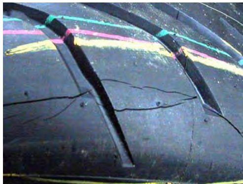
Tread cracking due to low temperatures
